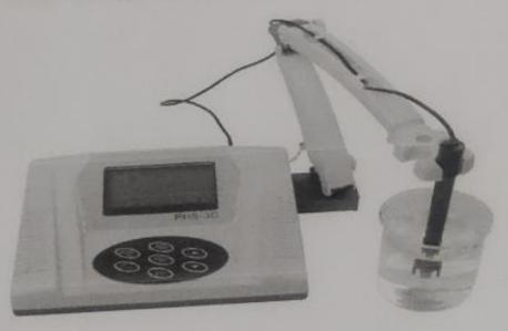
Procedure: Step1: We have to caliberate to remove errors with three types of solution(buffer solution) in 40seconds. Step2: Now we can test the pH of the sample.
